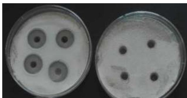
Evaluation of chemicals to inhibit bacterial growth. Left: inhibition zones of no bacterial growth developed around the agar wells filled with chemical A. Right: no inhibition of growth around agar wells filled with chemical B.
