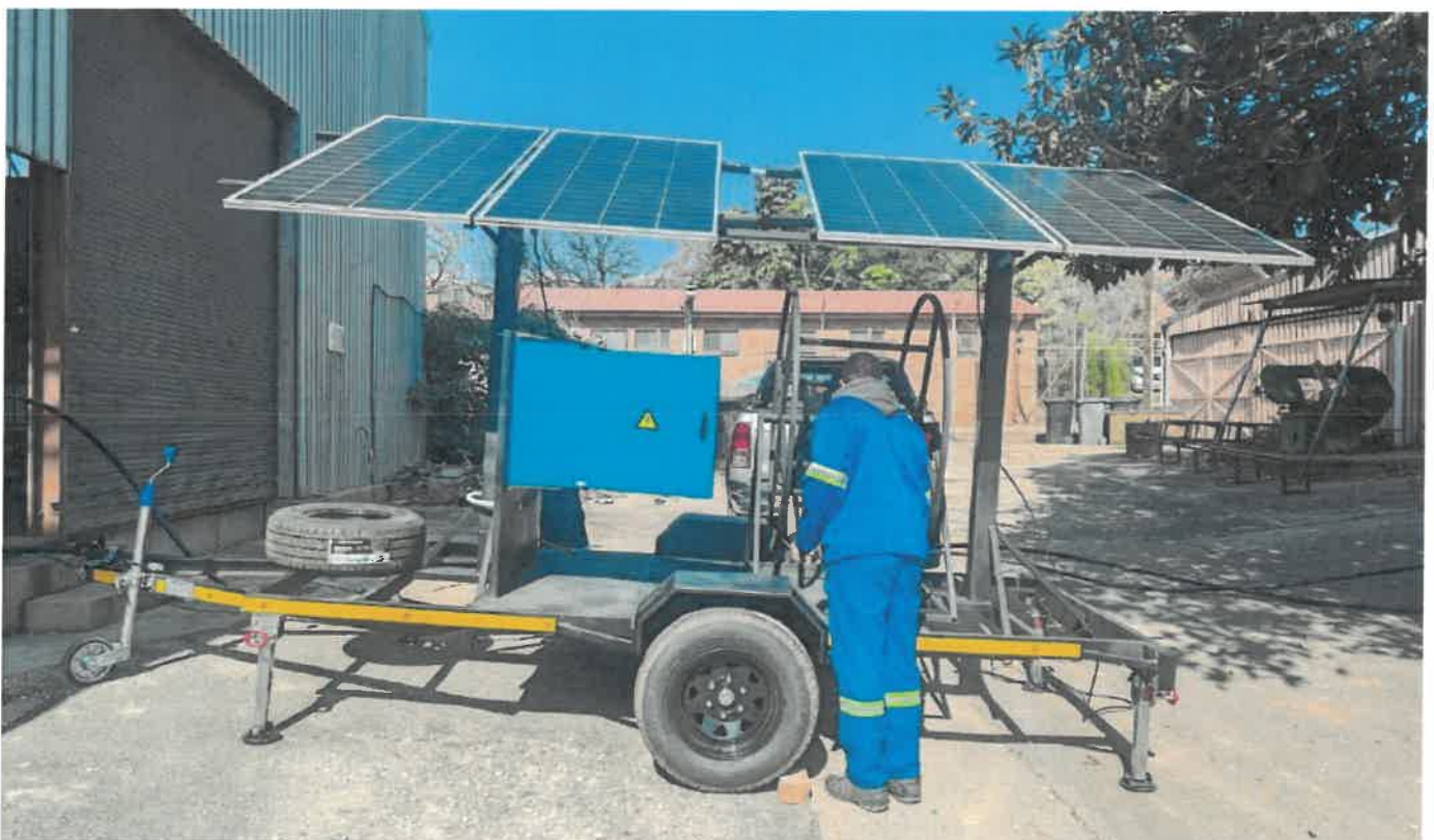
Figure 1 A mobile solar-powered system that supports on-farm water abstraction.
