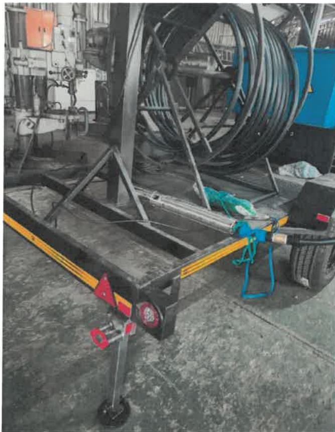
Figure 2 A mobile solar-powered trailer equipped with a submersible pump and piping system for portable water abstraction and irrigation support.
