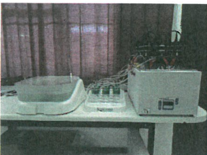
Figure 1: The ARC's biochemical methane potential testing system.
